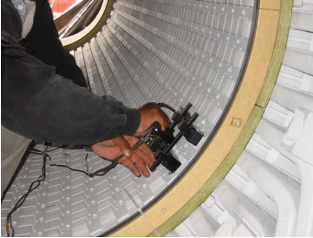
Figure 17.15 EI-CID trolley with Chattock coil mounted.
