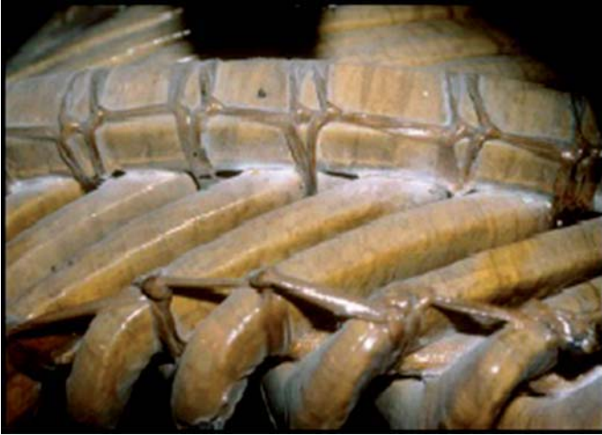
Figure 8.21 The white areas indicate fretting due to end winding vibration where the coils are lashed to a support ring in a motor stator.
