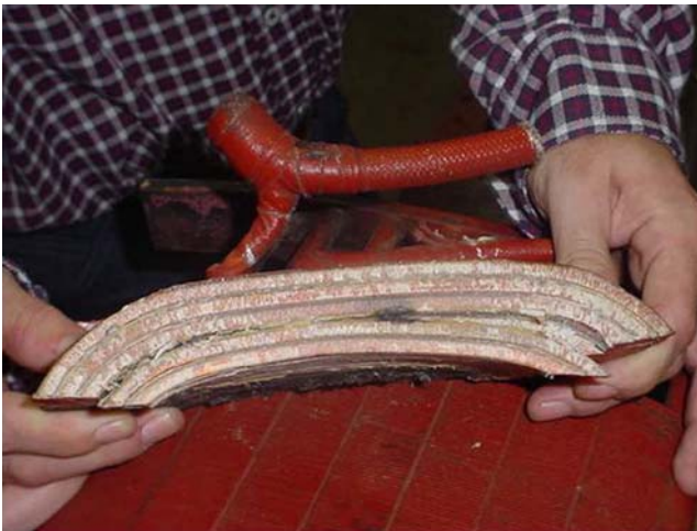
Figure 10.2 Turn insulation in wire wound coil resulting from cracking of the bonding resin as a consequence of thermal cycling.
