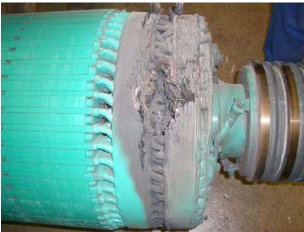
Figure 11.1 Rotor winding turn insulation failure from partial discharges.
