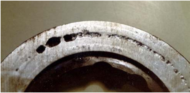
Figure 12.9 Voids in die-cast aluminum squirrel cage rotor winding (Source: Courtesy of EASA).
