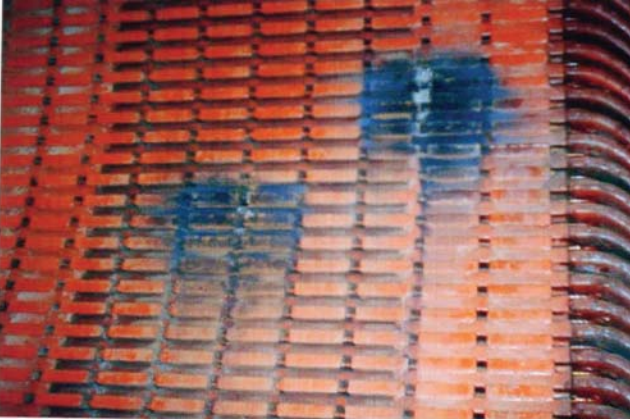
Figure 17.8 Thermographic image of core with damaged core insulation indicated by dark areas.
