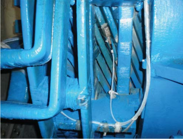
Figure 16.10 Photo of the installation of fiber-optic accelerometers on stator bars in an endwinding. (Source: Iris Power-Qualitrol.)
