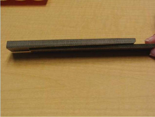
Figure 1.15 Side view of a two-part wedge, where a tapered slider is pushed under the wedge to increase radial pressure on the coils.
