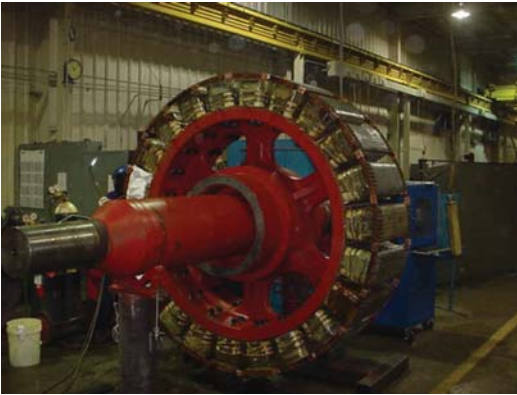
Figure 1.3 Photograph of a salient pole rotor for a large, low speed motor (Source: Photo courtesy of Teco-Westinghouse).
