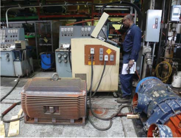
Figure 17.2 Commercial core tester exciting a motor stator core.
