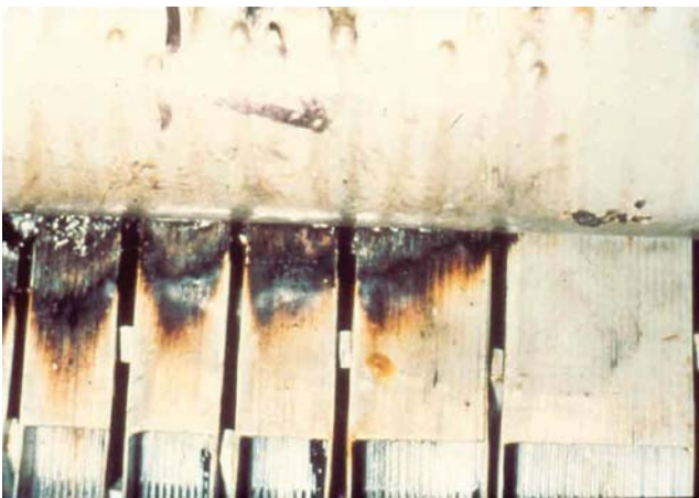
Figure 13.12 Back of core burning at key bar.
