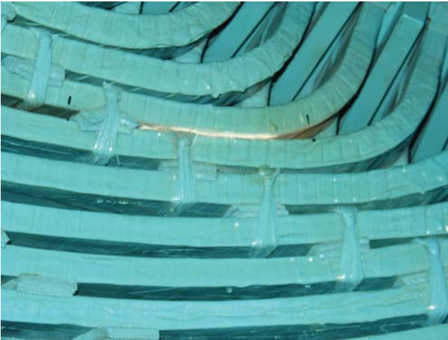
Figure 8.20 PD between adjacent coils in different phases results in white powder on the stator bar surfaces. (See color plate section).
