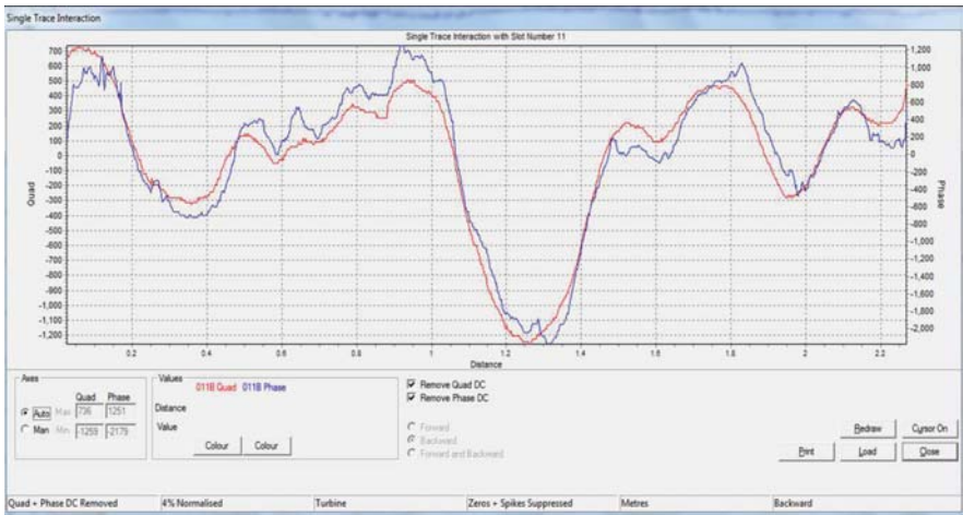
Figure 17.20 El-CID QUAD and PHASE current comparisons along a stator slot at a core split—same shape and constant PHASE/QUAD current ratio confirms that there is no core insulation damage. (Source: Courtesy Iris Power-Qualitrol.)
