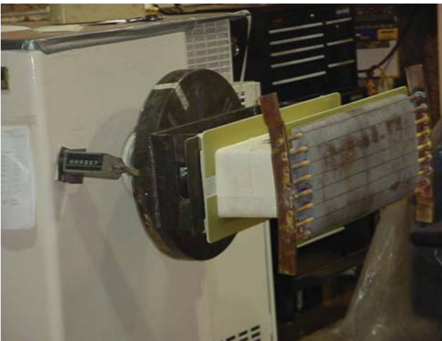
Figure 18.12 Resin-impregnated wire-wound pole windings.
