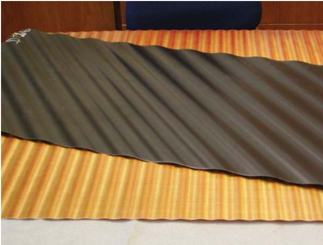
Figure 1.16 Photograph of semiconductive ripple spring material lying on top of nonconductive ripple sprint material (Source: Von Roll).
