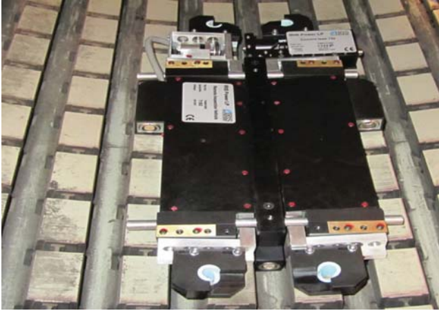
Figure 15.10 Photo of a wedge looseness detector mounted on a robotic vehicle to find loose wedges automatically in the stator. The detector is mounted in the middle, immediately over the wedges. (Source: Iris Power-Qualitrol).
