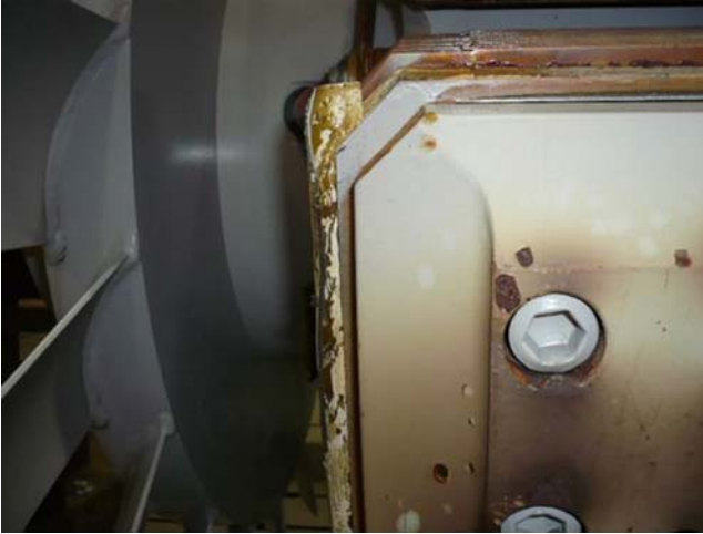
Figure 10.1 Strip-on-edge winding turn insulation migration from thermal aging of the bonding resin.
