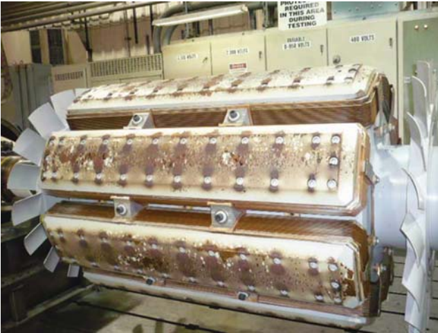
Figure 18.11 Laminated pole with ground insulation and pole washers installed ready for wire winding.
