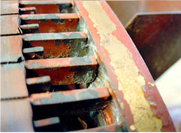
Figure 12.7 Rotor bar-to-shortening ring brazed joint failure due to poor manufacturing.
