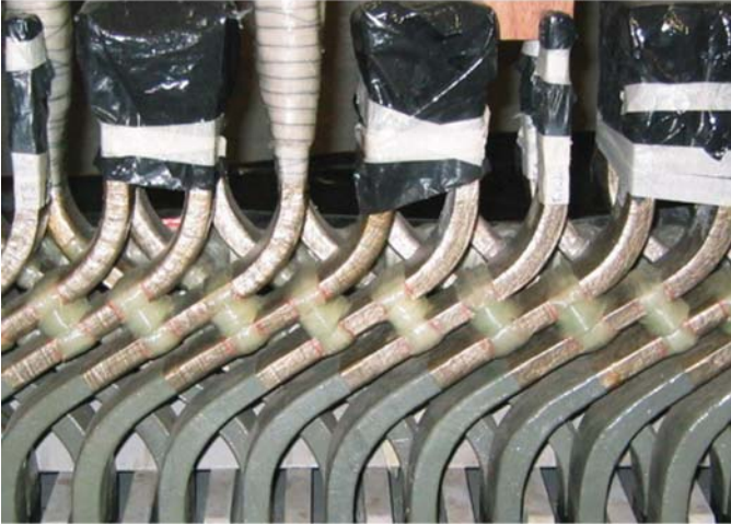
Figure 18.1 Interbar blocks covered with felt.
