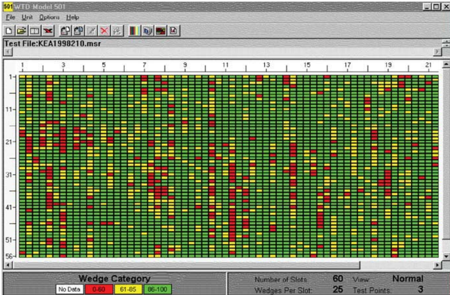
Figure 15.9 Map of wedge tightness versus slot number (vertical scale) and axial wedge number (horizontal scale). Green is tight, red is loose, and yellow is indeterminate. (Source: Iris Power-Qualitrol).
