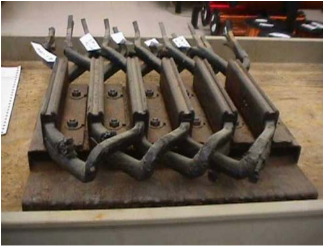
Figure 2.2 Photograph of a formette containing four multi-turn coils after a thermal endurance test (Source: Eltek Laboratories).
