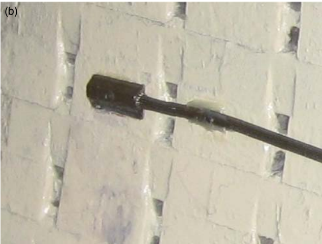
Figure 16.13 (a) A photo of a conventional wedge-mounted foldable flux probe that projects into the air gap. (b) A photo of an installed flat flux probe glued to a stator tooth. (Source: Iris Power-Qualitrol.)
