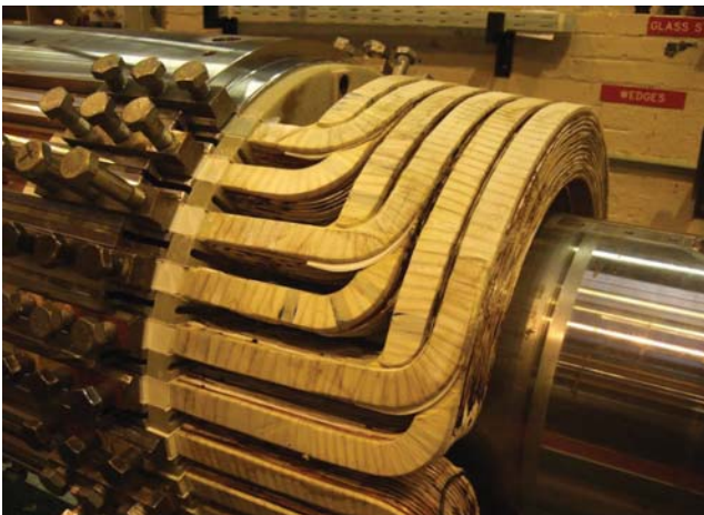
Figure 18.6 Round rotor field winding top turn taping.
