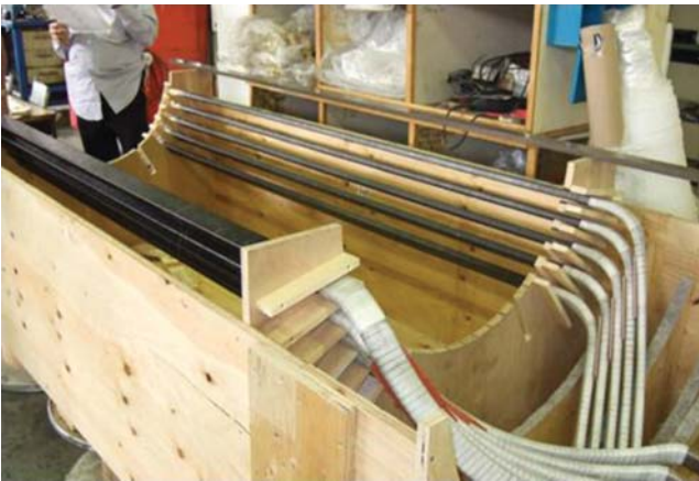
Figure 18.3 Stator core mockup to check bar fit and endwinding spacing.
